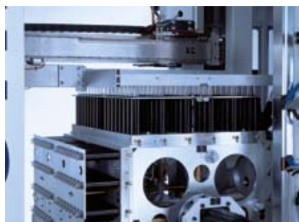
above: 96 cav. vertical 4 station post mold cooling below: 96 cav. horizontal 3 station post mold cooling
