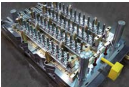
Refurbished cold half
