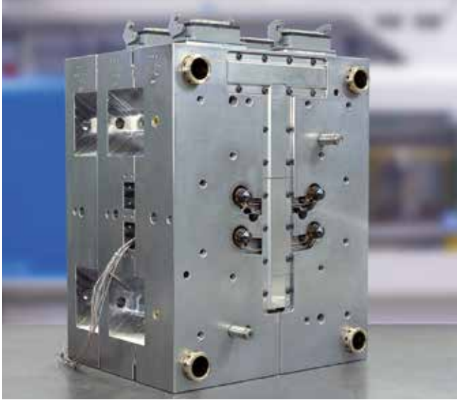
Fig. 1. Hot runner of the test mold with three platens to simulate the length of the melt runners in a 96-cavity mold (© MHT)
