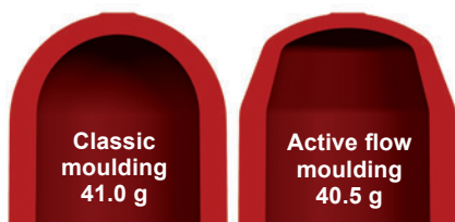
Comparison: conventional round base (left) and Antiflex base (right)
